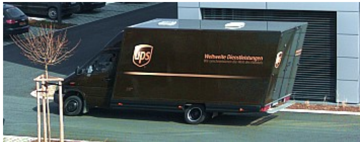
Example for the rolling shutter effect with a moving car
